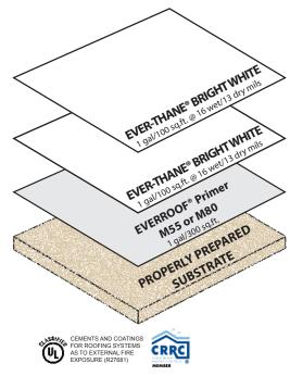
EVER-THANE BRIGHT WHITE is a versatile, multi-purpose, aliphatic, single-component, moisture-cure, urethane coating designed for use as a top coat or for repair work on metal and other roof systems.
